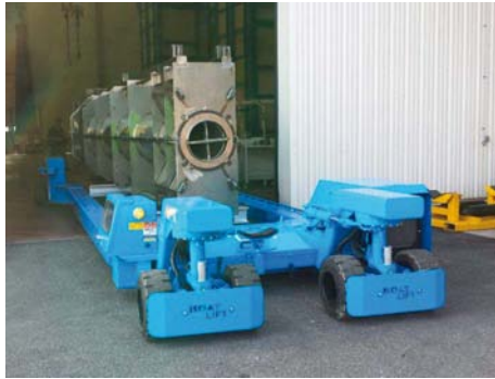
Industrial Lift 10 ton in France Used to move steel moulds for plastic injections
