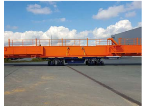
Industrial Lift 80 ton in Germany Used to move overhead bridge crane
